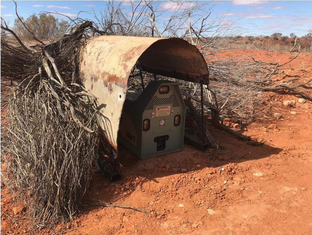
Felixers are stationary devices equipped with sensors, a camera, and a delivery mechanism that fires a measured dose of poison onto the fur of a target animal, which is subsequently ingested through oral grooming.
